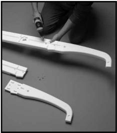
**#1:** Overlap the flat end of the Handrail onto the top of the Side Rail. Using two  $1/4 - 20 \times 5/8$ " bolts and two 1/4 - 20 hex nuts, attach the Handrail to the Side Rail. Repeat for the remaining three Side Rails.
