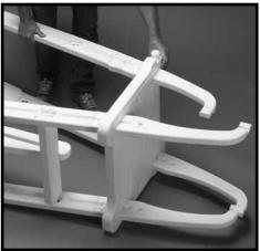
**#1:** Flip entire ladder assembly onto its side. Slide the two remaining Side Rail assemblies through the two openings on the tabbed end of the Platform. Using the rubber mallet, tap down on the Platform until it is seated against the lugs
