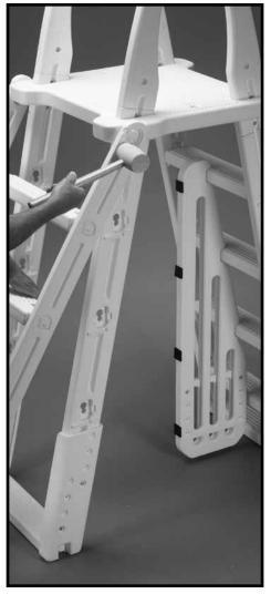
**#5:** Using the rubber mallet tap down to secure.
