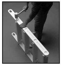
**#3:** Place the remaining Swing-up Rail over the tabs of the Swing-up Treads and tap into place using the rubber mallet. Set this assembly aside.
