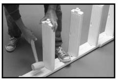
**#3:** Placing your foot on the Side Rail to hold it steady, use the rubber mallet to tap down the Fixed Ladder Treads until they are firmly seated in the Side Rail.
