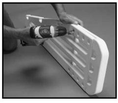
**#2:** Position the Anti-Swim Barrier Extension over the Anti-Swim Barrier rier so that the length of the Barrier matches the length from the top tread to the bottom tread of the ladder. Attach with two 1/4 - 20 x 1 1/4" bolts and two 1/4- 20 hex nuts.
