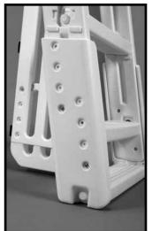
**#3:** Check to make sure the hole locations in the platform are clear of pool wall and supports. Drill two 5/16" holes through the Platform and pool ledge. Fasten the ladder platform to the pool ledge using two 1/4-20 x 2-1/4" bolts, 1/4-20 hex nuts. You MUST secure the ladder to the pool top rail for strength and stability.
