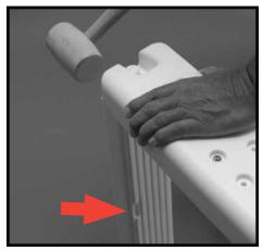
**#3:** Position the remaining Fixed Ladder Tread so that the tabs align with the notches at the bottom of the Side Rail assemblies and tap in with the rubber mallet until the tread is properly seated. NOTE: The small groove should face the inside of the ladder.
