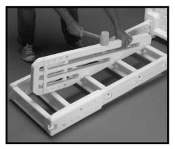
**#3:** Using the rubber mallet, tap the Anti-Swim Barrier into place.
